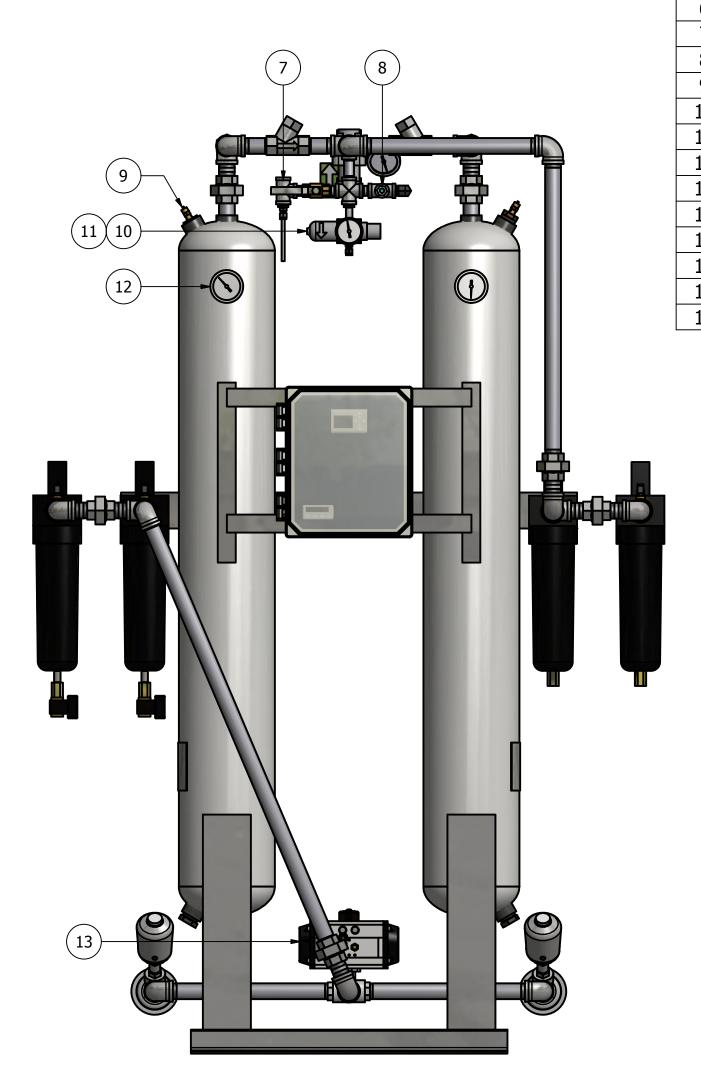
PRESSURE REGULATOR, PURGE 2 PRESSURE GAUGE, PURGE 3 1 CHECK VALVE, PURGE 2 4 SOLENOID VALVE, REPRESS 5 1 COALESCER PRE-FILTER 6 2 DEW POINT MONITOR (OPTIONAL) 7 1 MOISTURE INDICATOR 8 1 2 RELIEF VALVE, TANKS 9 10 PRESSURE REGULATOR, CONTROL PRESSURE GAUGE, CONTROL 11 1 12 PRESSURE GAUGE, TANKS 2 13 1 3- WAY BALL VALVE, INLET PARTICULATE AFTER-FILTER 14 2 ANGLE BODY VALVE, EXHUAST 15 MUFFLER, EXHAUST 16 2 MANUAL BALL VALVE, BYPASS 17 9 18 120 LBS DESICCANT
